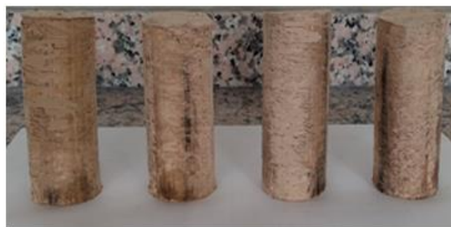
Figure 5. Reinforced with basalt fiber cylindrical samples prepared for unconfined compressive test
