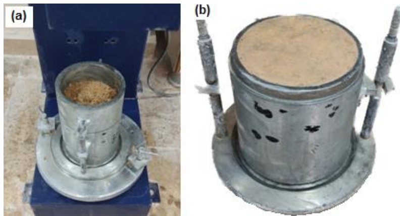
Figure 4. Performing the standard proctor test (a), compressed sample as a result of the test (b)
