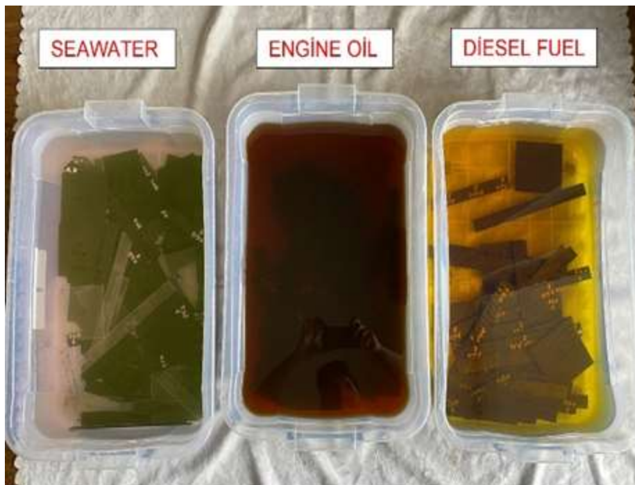
Figure 3. The process of placing composites into degradation environments.
