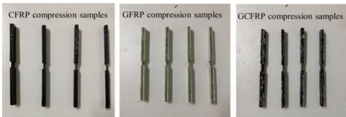
Figure 4. Compression samples of CFRP, GFRP and GCFRP composites.
