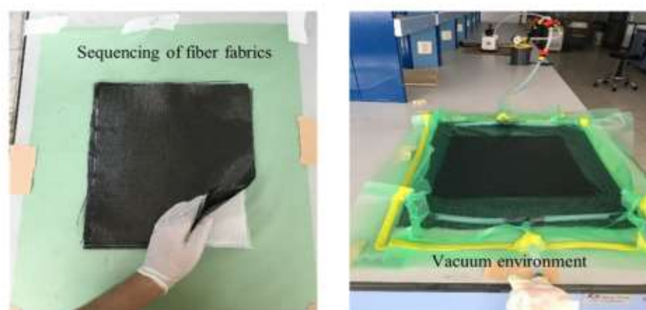
Figure 2. Processes of producing composites with VARTM method.
