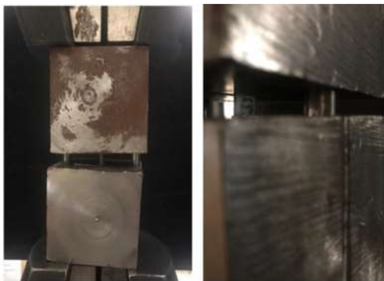
Figure 5. Application of compression test on composite specimens.
