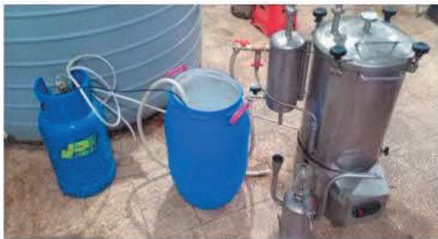
Figure 1 Hydrodistillation method for extraction of essential oils
