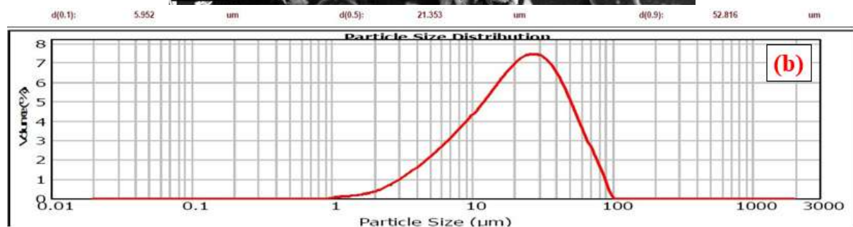
Figure 3. (a) Morphology (b) Particle size distribution of graphite particles
