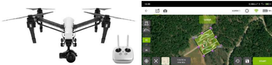
Figure 2. a) DJI Inspire I UAV (left) b) Flight path created with Pix4Dcapture (right).
