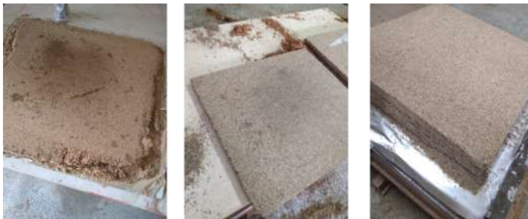
Figure 4. Particles boards with different almond shell particle volumetric ratios, just released from the molds.
