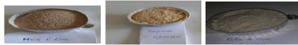
Figure 1. The different loadings filler used (olive nuts, sawdust and waste glass / unsaturated polyester composites) of fine size ( \leq 500 \mu\text{m} ).
