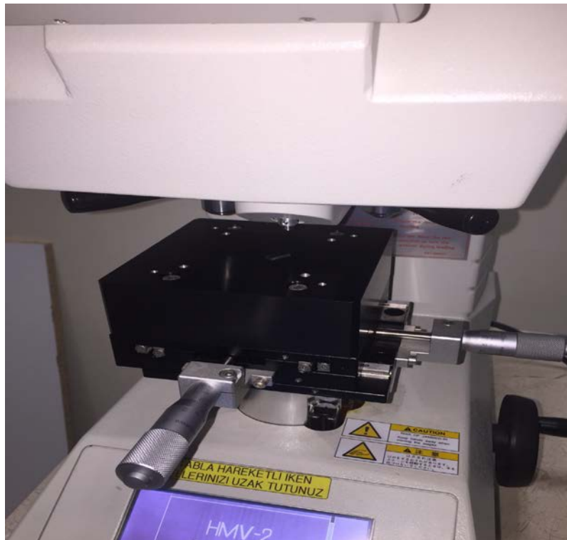
Figure 1. Measurement apparatus of SHIMADZU HVM-2 model digital tester
